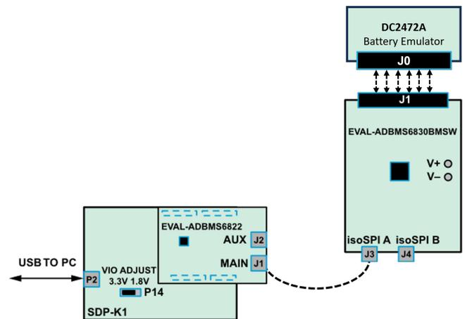
Figure 2. Cell Monitoring Setup
