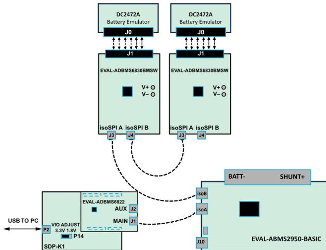
Figure 5. Complete Daisy Chain Setup
